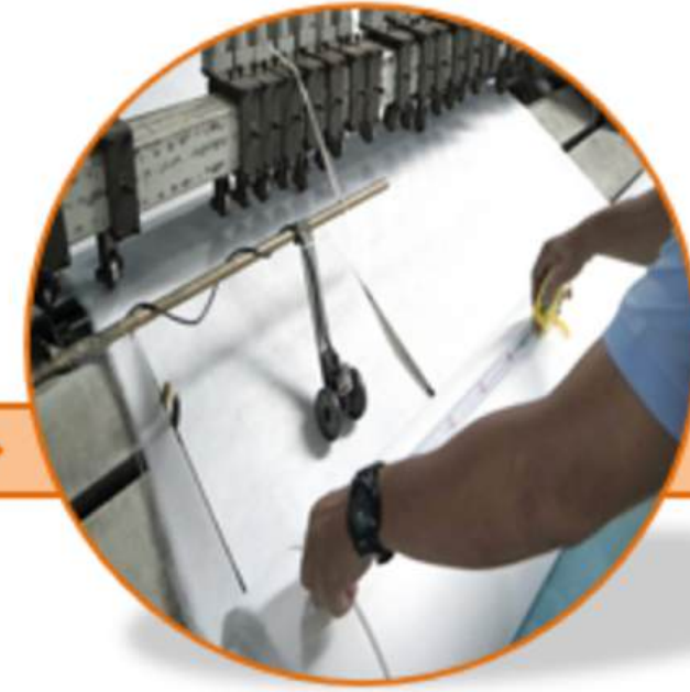
Checking the width on the fabric surface
